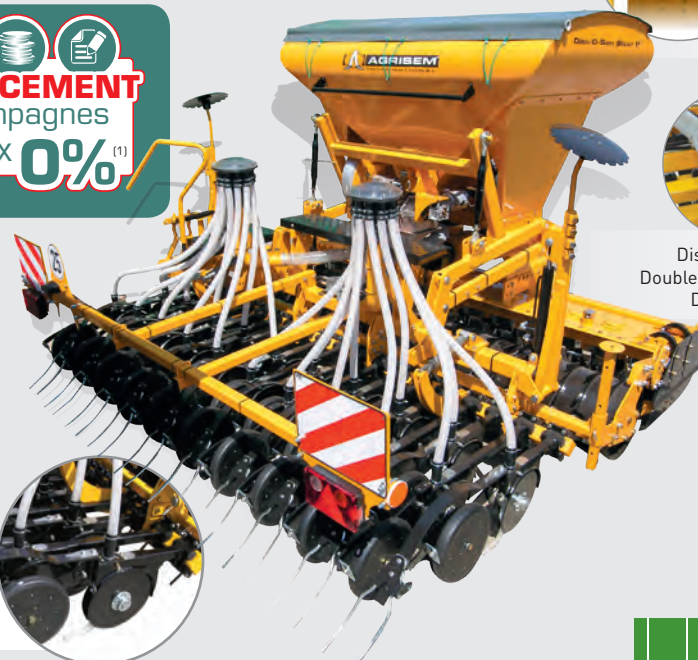
Rampes de semis "minimum tillage" Pression 120 kg/élément
